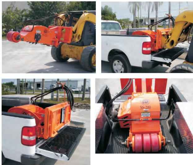
The SS-200 makes easy work of maintenance and storage. Along with periodic lubrication and conformity to warranty guidelines, the SS-200 will give you many years of trouble-free and profitable use. Because of its unique compact design, it can also be quickly transported on the back of any 1/2 ton pick up truck.
